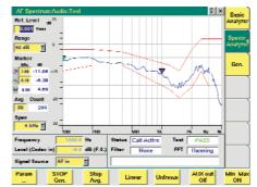
The audio template allows thorough testing of frequency responses from mobile phones. A simple PASS/FAIL allows a quick check of the mobile's performance. The template can be created and saved by the user depending on the test set-up used.
