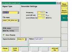
AF generator provides for different frequency and level settings or for multitone the usage of wavefiles. The audio signal can be sent either to the AF out, the codec input (internal) or to the auxiliary connector.
